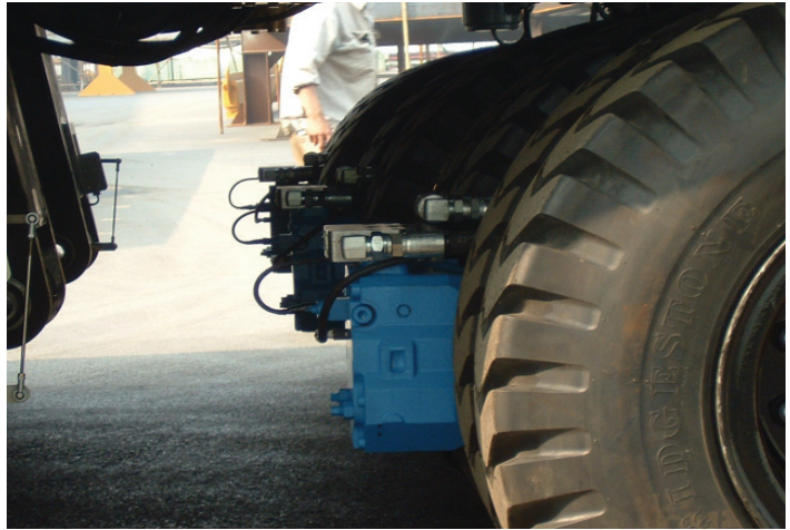
Eaton DuraForce pumps, motors, and valves are equipped on the trailer's hydraulic system that powers 18 axles.
